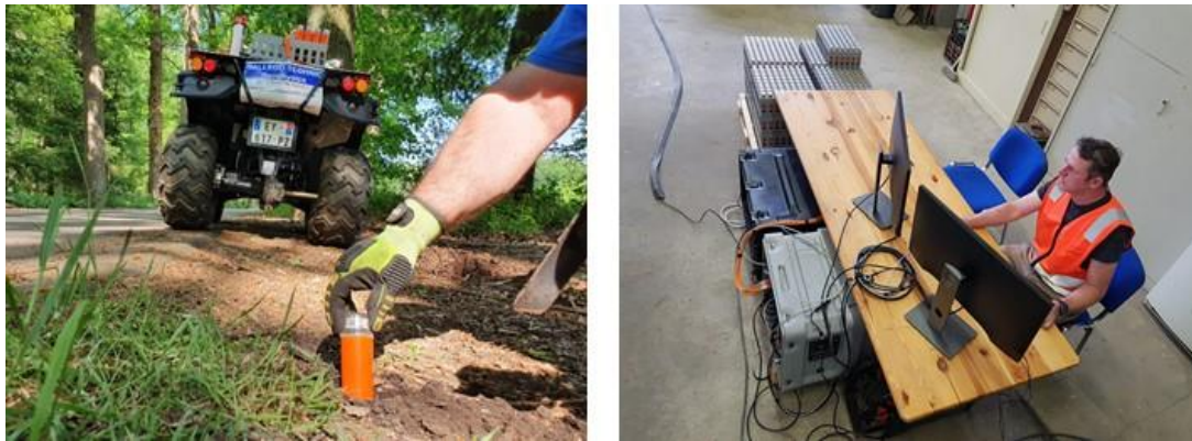
Figure 1 Exemple of deployment of STRYDE nodes for the 2D test. Light field system for the deployment and harvesting of the nodes
