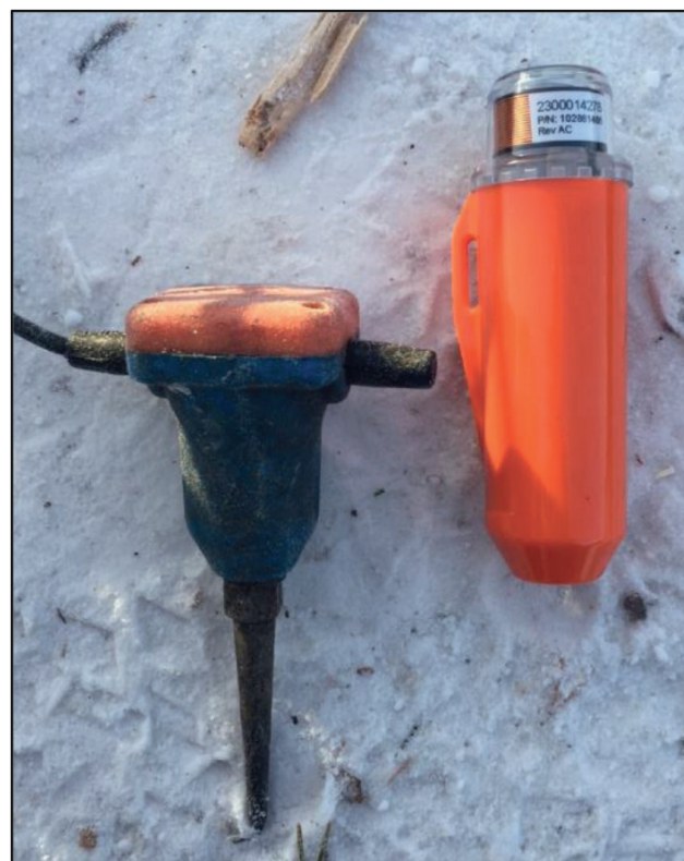
Figure 5 Comparison of Nimble Node and a single geophone (each group had 12). Note reduction in equipment weight and complexity with the nodal system.
