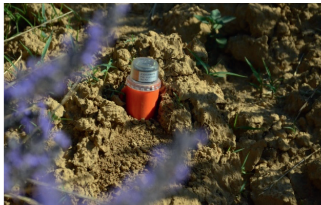
Figure 7 STRYDE node deployed in the ground.
