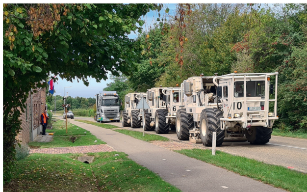
Figure 4 The three Mertz M12 VibroSeis trucks in the same area in 2022, as comparison.
