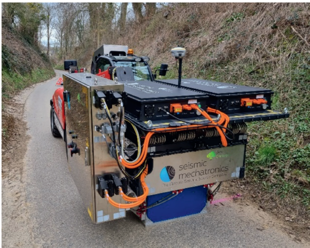
Figure 2 Battery-powered Storm 10 eVibe during production.
